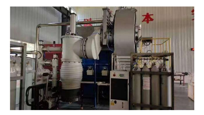
The large-scale PREP equipment (SLPA-N75) is purposely designed for continuous, industrial mass production of high quality spherical Titanium alloy powders with the following characteristics:
